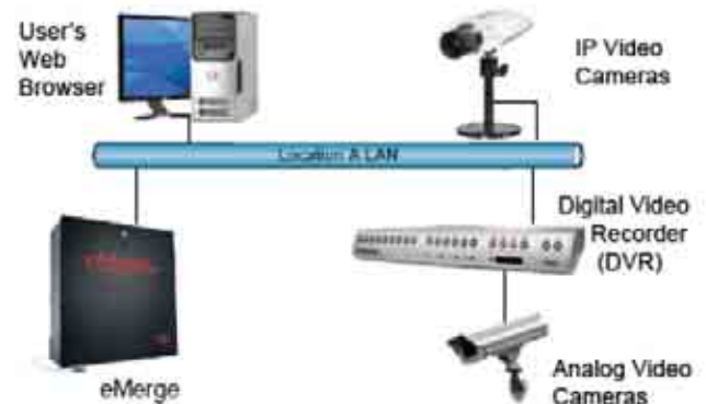
All components are connected to the network. Both IP and analog cameras are supported
